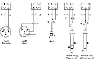
INPUT/OUTPUT CONNECTOR WIRING DIAGRAMS Figure 8
